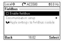
Use the settings in the **Fieldbus** submenu to use the drive with a fieldbus:
