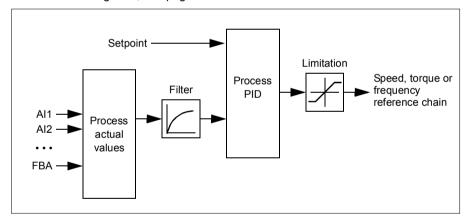
The drive contains two complete sets of process PID controller settings that can be alternated whenever necessary; see parameter 40.57 PID set1/set2 selection.
