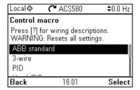
Use the **Macro** submenu to quickly set up drive control and reference source by selecting from a set of predefined wiring configurations.
