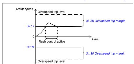
whenever the motor speed exceeds 30.11 Minimum speed or 30.12 Maximum speed.
