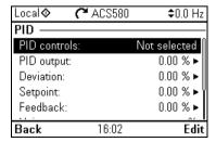
The PID submenu contains settings and actual values for the process PID controller. PID is only used in remote control.
