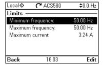
Use the **Limits** submenu to set the allowed operating range. This function is intended to protect the motor, connected hardware and mechanics. The drive stays within these limits, no matter what reference value it gets.
