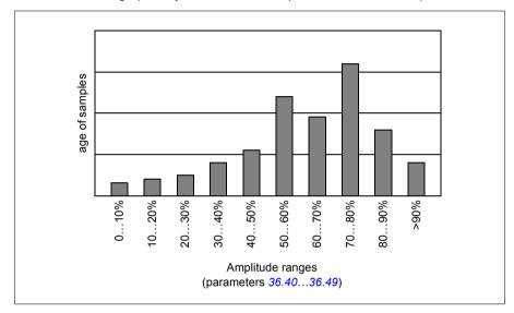
Amplitude logger 1 is fixed to monitor motor current, and cannot be reset. With amplitude logger 1, 100% corresponds to the maximum output current of the drive  $(I_{\text{max}})$ . The measured current is logged continuously. The distribution of samples is shown by parameters 36.20...36.29.
