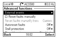
The Advanced functions submenu contains settings for advanced functions, such as triggering or resetting faults via I/O, or switching between several entire sets of settings.
