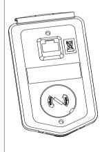
To reinstall the control panel, put the bottom of the container in position (1a), press the retaining clip at the top (1a) and push the control panel in at the top edge (1c).
