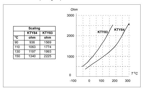
It is possible to adjust the motor temperature supervision limits and select how the drive reacts when overtemperature is detected.
